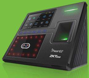
iFace402 multi-biometric identification Time & Attendance and Access Control terminal adopts ZKTeco's latest platform with ZKFace algorithm and large capacity memory. With the upgraded hardware, it can now store up to 1200 face templates.
