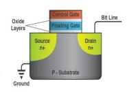
Figure 6: Diagram of a flash memory cell, which stores data as a charge on a "floating" gate.
